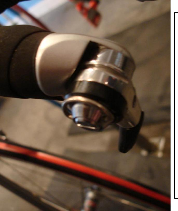
Be sure that the shifter is still in the last gear with the least amount of tension on the cable to allow the derailleur to drop as far as it can into the proper position. Next is to adjust the Low Limit Screw. This screw is located as the lower of the two screws and typically labeled above with a "L" above it.
