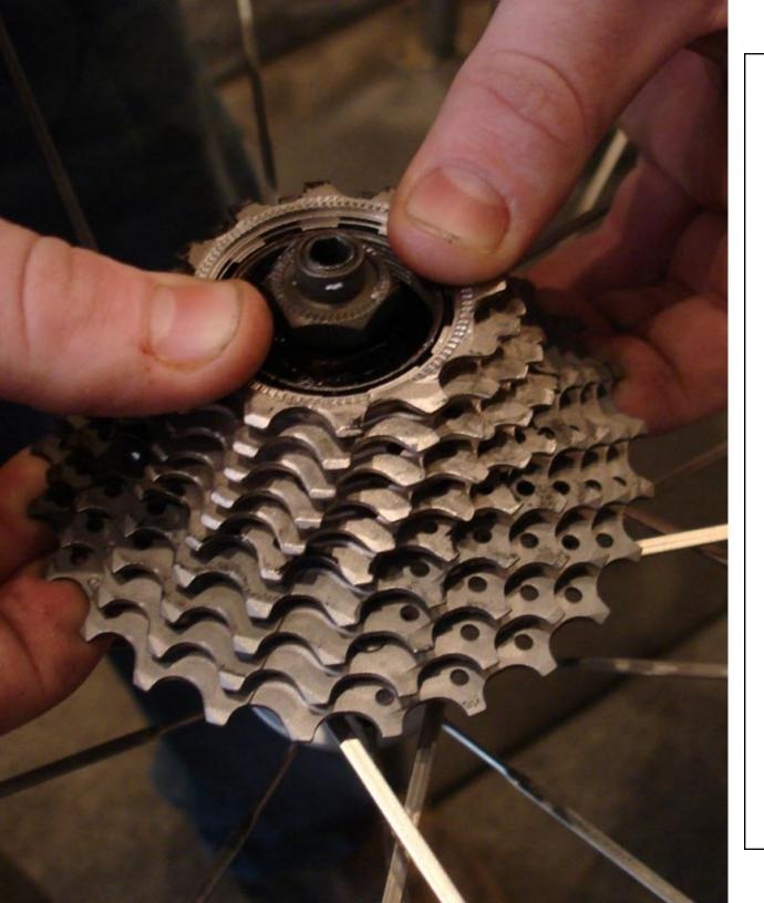
As the lockring has been taken off, put the wheel horizontal and grab the entire cassette. The whole cassette should come off altogether. If the cassette feels sticky, it can be removed one cog at a time to find the one stuck, as sometimes cogs dig into the hub cassette body. This may be able to be removed by putting a flat head screw driver between the cogs and turning it to pop the cog free.
