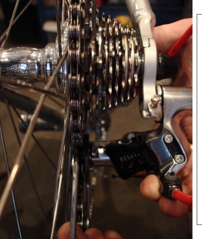
Adjust this screw in or out to have the top pulley on the derailleur line up with the last cog on the cassette.
