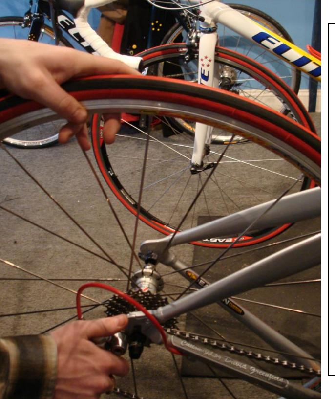
Here you see the derailleur out of the way while the wheel is coming out of the drop outs as to not scratch or interfere with one another.
