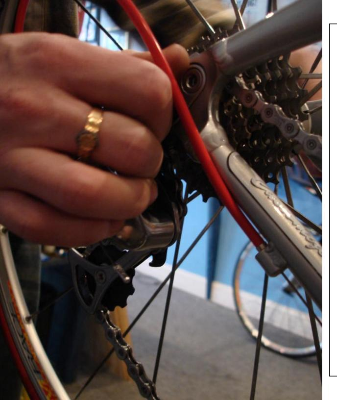
After the wheel's brake is open move to the skewer and release the handle while holding onto the wheel to have control over the wheel while taking it out of the dropouts.
