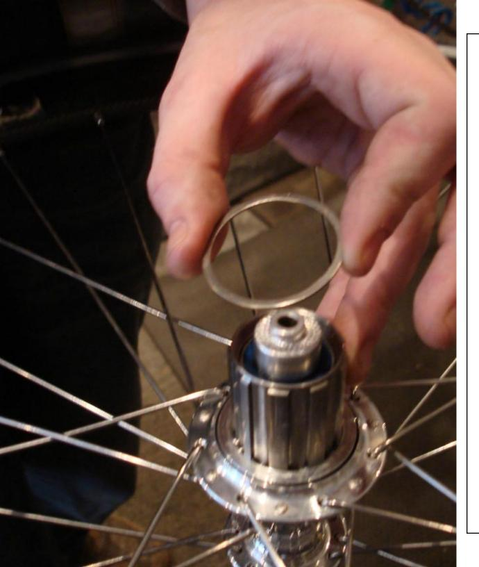
First thing to go onto the race wheel is the thin steel spacer that should be able to just fall onto the cassette body.
