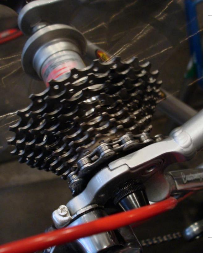
After shifting make sure to pedal so the chain drops all the way into the last cog to have the rear derailleur the furthest from the wheel to enable the most ease to release the wheel.
