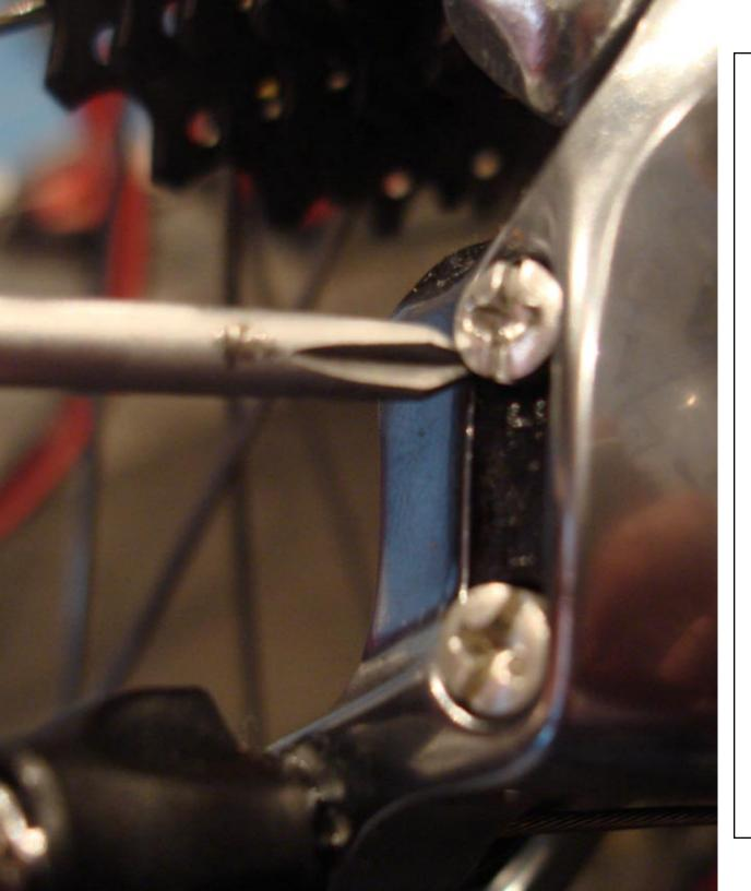
The High Limit Screw is labeled with an "H" under it or typically located as the top screw. If this is questionable look inside the derailleur itself to see which of the two screws is being touched while in the high gear.
