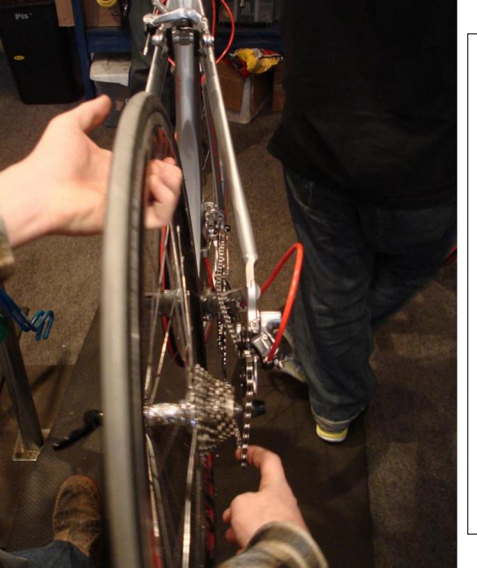
Starting as ended from taking the rear training wheel out will put the race wheel in. Pull the chain down to ease the cassette in between it but not to catch a cog on the bottom.
