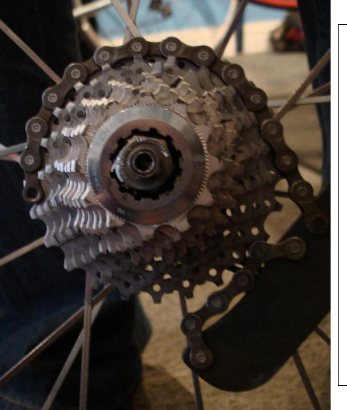
This is how your chainwhip should fit on your cassette. Make sure to put as much of the chain over the second to largest cog. This is to give the chainwhip as much torque on the cassette while not having the possibility of the chain running into the spokes. Also note that the tool should be in your left hand while the wheel is facing away from you.
