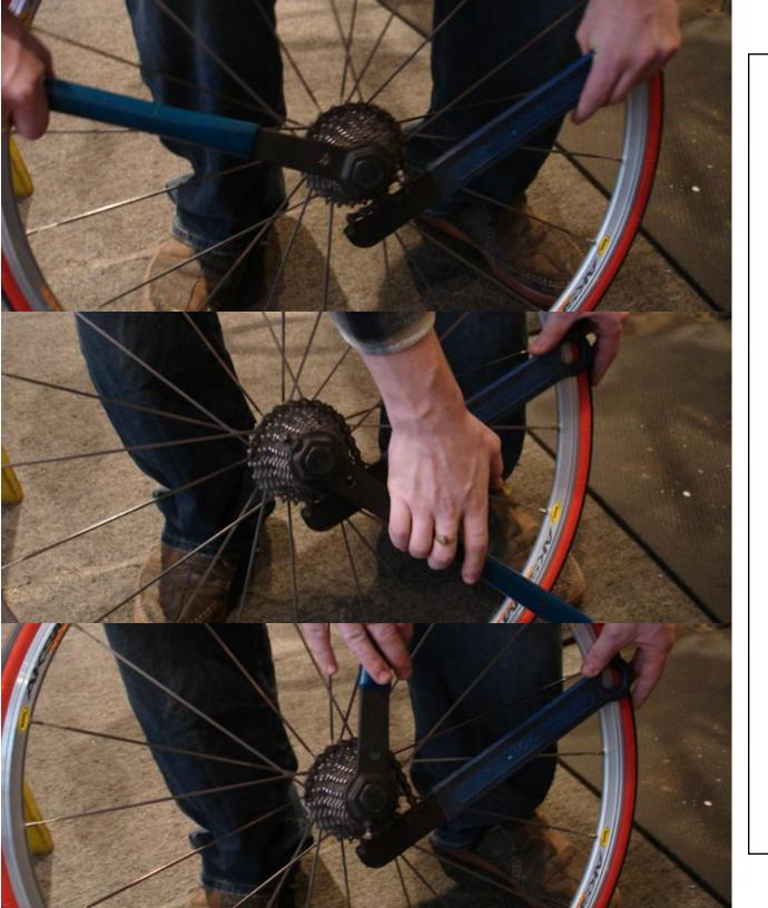
After both tools are on the cassette, hold the chainwhip while pushing down on the lockring tool and spinning off the lockring.
