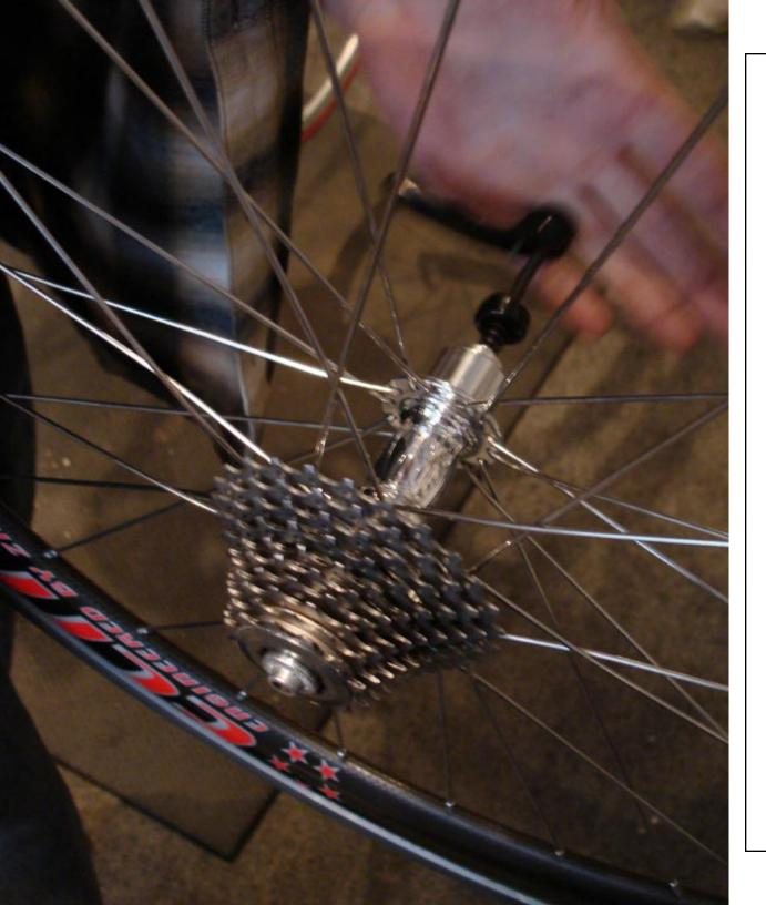
Take your skewer from the training wheel, unless you have a race skewer and slide back through the wheel with the handle on the non-drive side of the wheel. Make sure there is grease on the skewer and its threads to prevent it from freezing from sweat and elements affecting the skewer.
