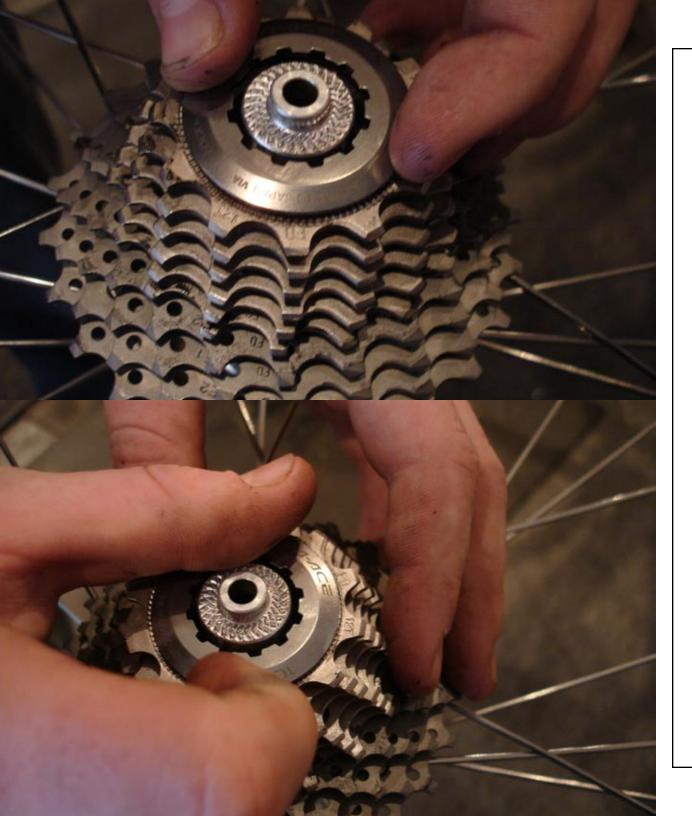
Once the cassette is on the lockring can be hand tightened into the hub body cassette to hold the cassette in place. Make sure to put the lockring on by hand to prevent from cross threading the few threads available on the lockring.
