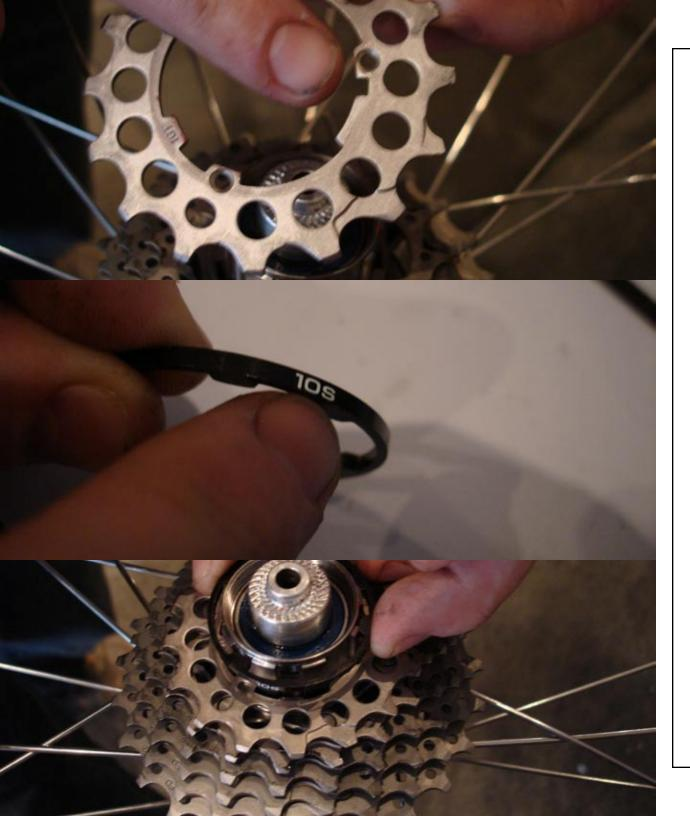
On a Dura-ace ten speed cassette the next few have separate spacers from cogs. It starts with the next cog, then a spacer that is labeled "10S" for ten speed cassettes. This is how the cogs should be coming along, biggest to smallest.
