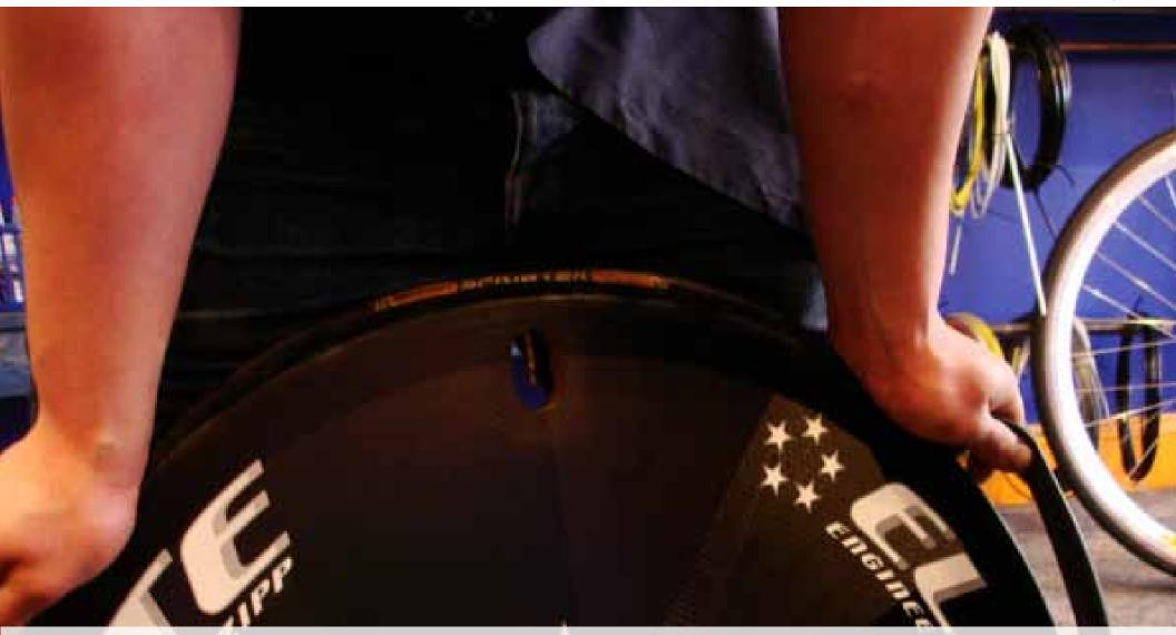
After placing the valve in straight, put equal pressure down heavily on the tire stretching tire over the rim. The more pressure you put in the beginning, the less you will have to use to get the last part of the tire on.
