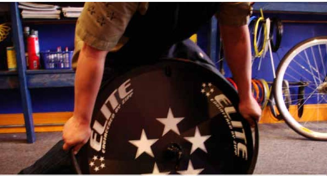
Keeping pressure continually along both sides of the rim it is a good idea to lean the rim against your leg and crouch to get better leverage on keeping pressure on the stretching the tire.
