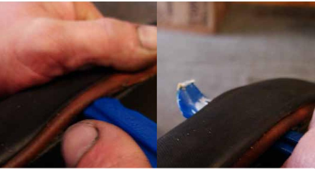
After getting the tire lever under the tire, continue to push back and forth to pull the glue away from both of them, and pull tire to the side using leverage with the tire lever to get the tire coming off the rim to be able to grab it by hand.
