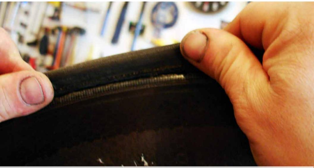
After the tire is on the entire rim, proceed to center the tire on the rim before inflating. The cloth tape on the tire should be showing on both sides of the rim about 3 mm. Check one side and flip the wheel to see if it is even on both sides.
