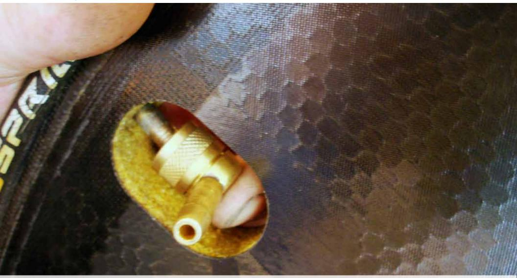
The next step is getting the angle pump adapter onto the valve of the disc.
