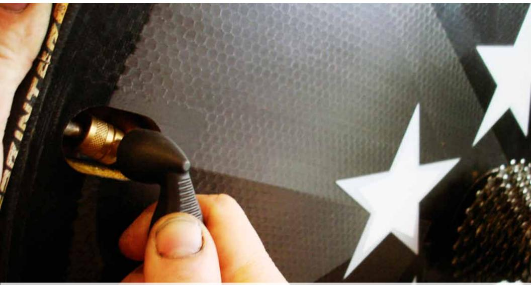
Next simply attach the nozzle of the inflator onto the adaptor and slightly unscrew the canister to inflate the tire
