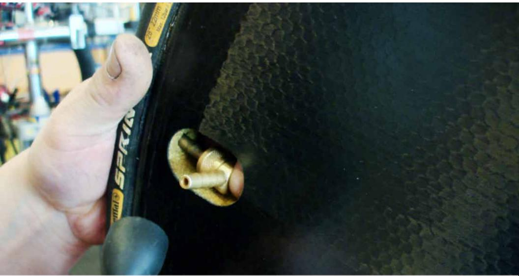
Once the tire is inflated you can remove the inflator from the angle pump adaptor. This will not effect the air in the tube from coming back out.
