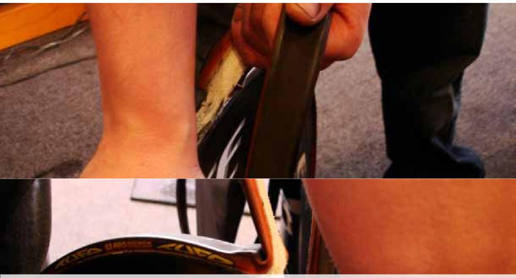
After getting the tire down beyond half the wheel, can then pull the tire off of the rim each way to rip towards the valve hole.
