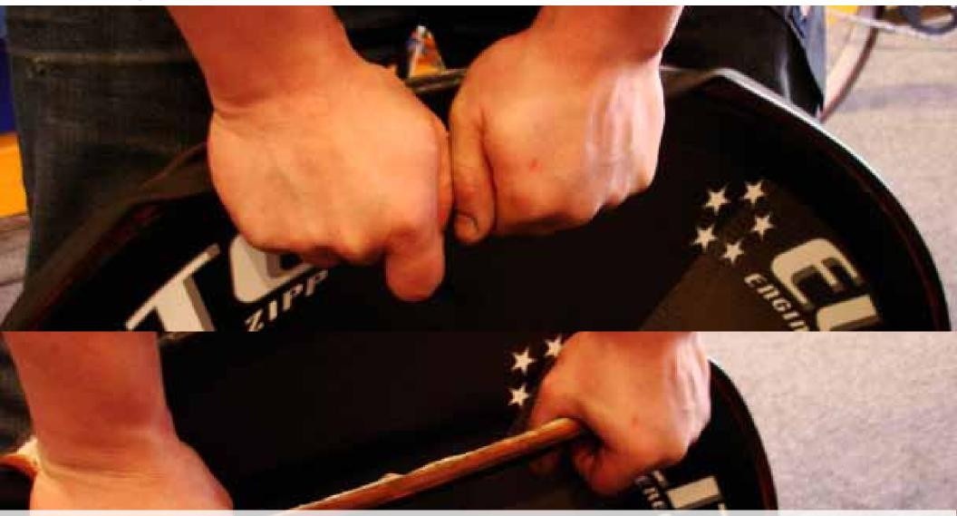
After getting the tire this far, can then stand over the wheel and use weight and force to start ripping the tire down towards the ground.
