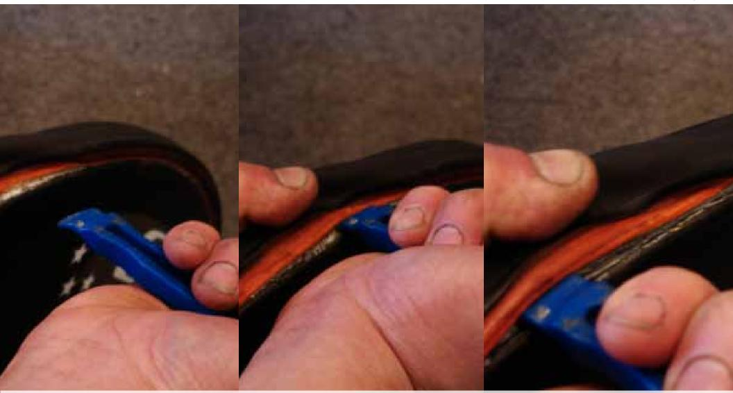
First, once you get a flat, downshift the bike to your hardest gear to allow the wheel to come out of the dropout easier(and also easier when putting it back in later). Then, after getting the wheel out take tire lever with somewhat of an edge on it and pull the tire back and run the tire lever back and forth to break up the glue "threads" showing to get the lever between the tire and the rim itself.
