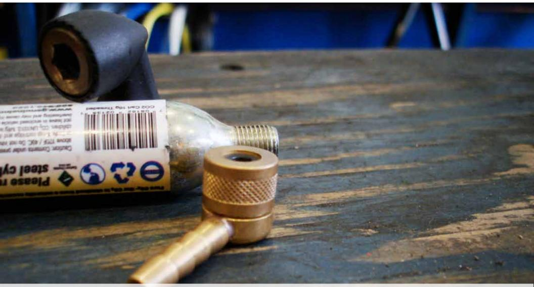
In this case we will be using an angle pump adapter for usage on discs and some other carbon wheels this will be needed.
