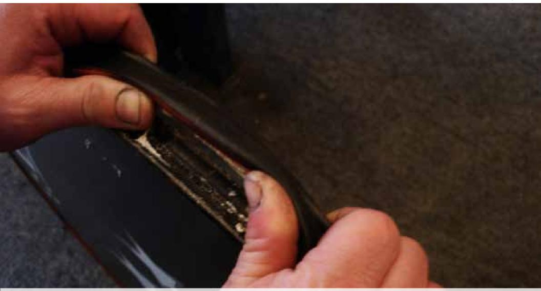
Getting the glue to let go of holding the tire on the rim by bending it back and forth against the direction of the rim and gain more and more leverage.
