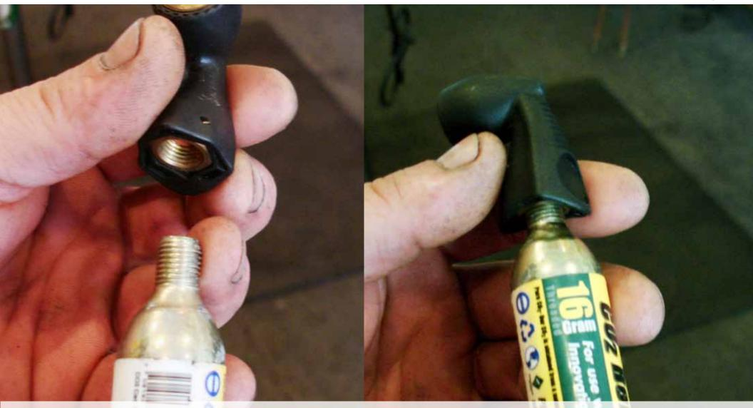
If you have never used a CO<sub>2</sub> inflator before, screw the inflator onto the canister, this will pierce the tank, which stays closed, then to release the air unscrew the cap slightly.
